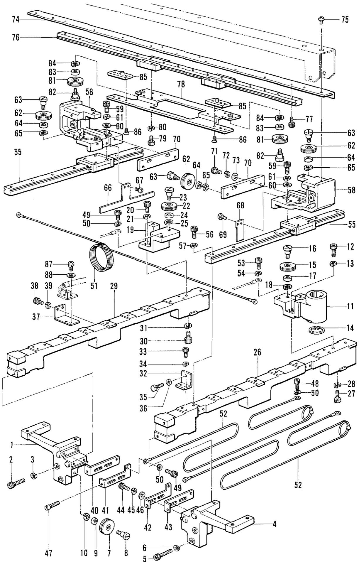
M. 送り・案内関係/Feed guide mechanism/Transportführung/
