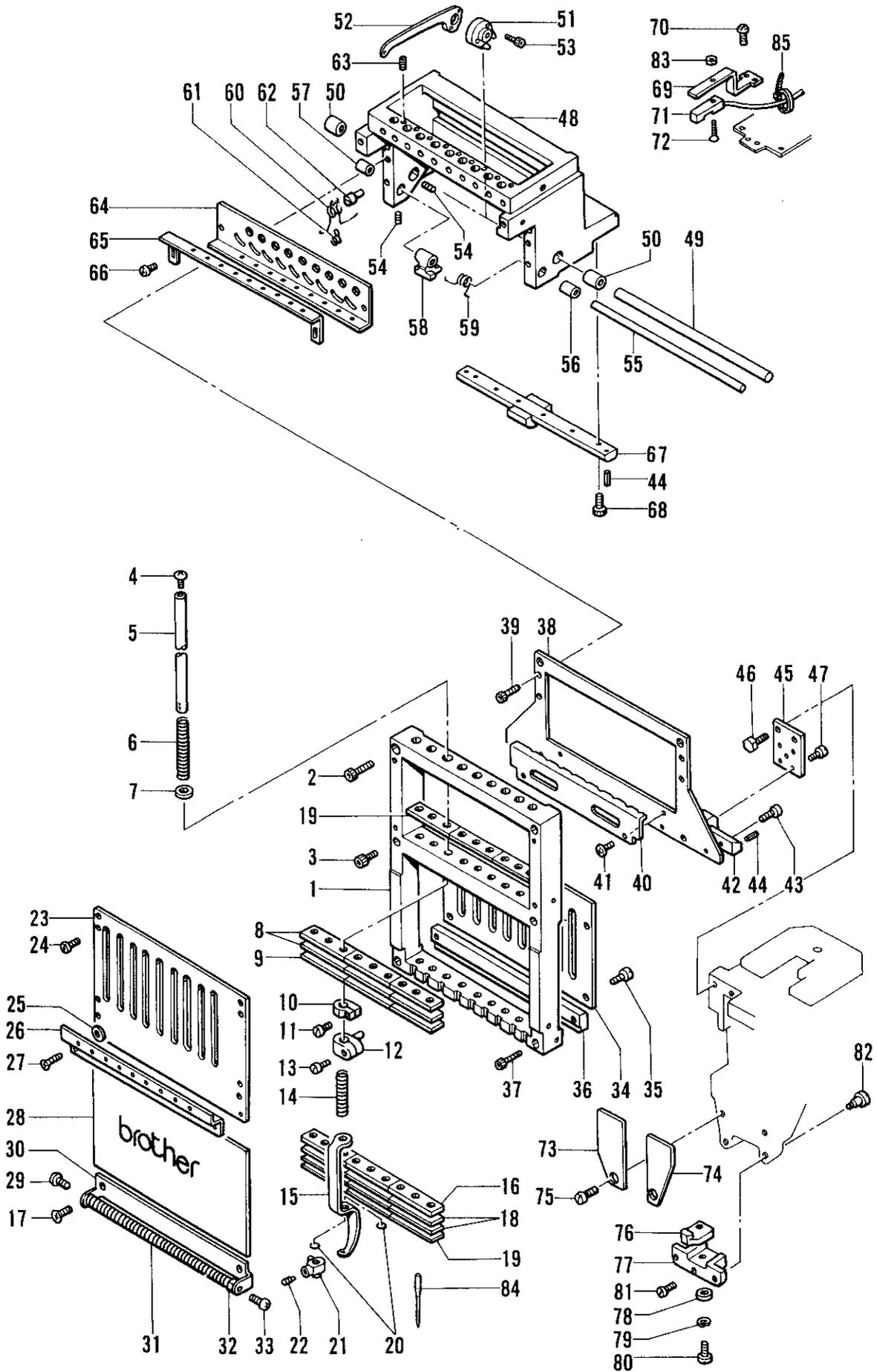
B. 針棒関係/Needle bar mechanism/Nadelstangenvorrichtung/
