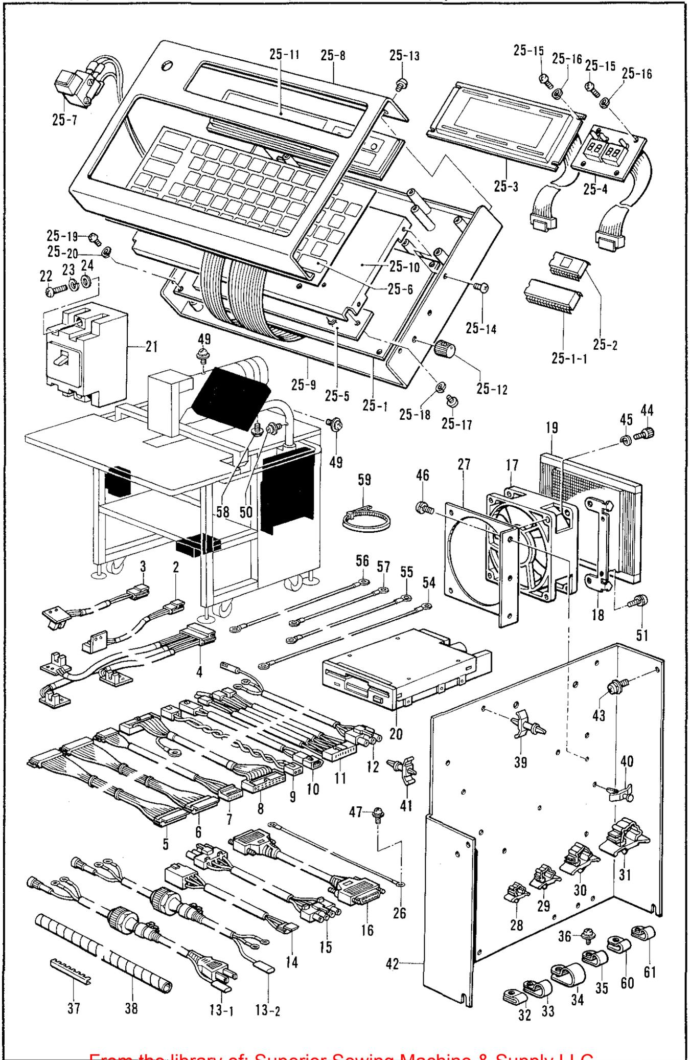
R2. 電装品関係 / Power supply equipment mechanism / Stromversorgung / Mécanisme
