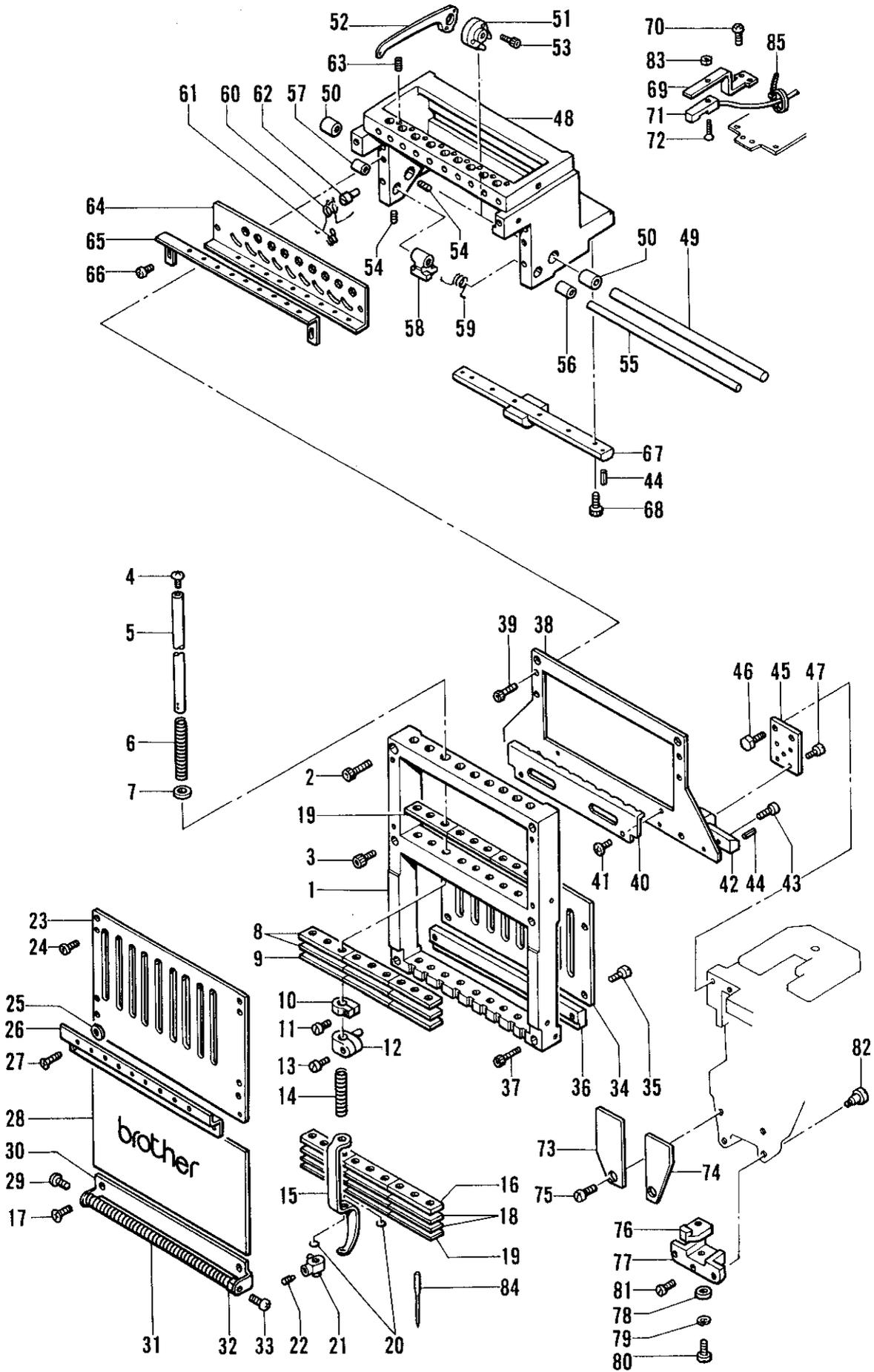
B. 針棒関係/Needle bar mechanism/Nadelstangenvorrichtung/
