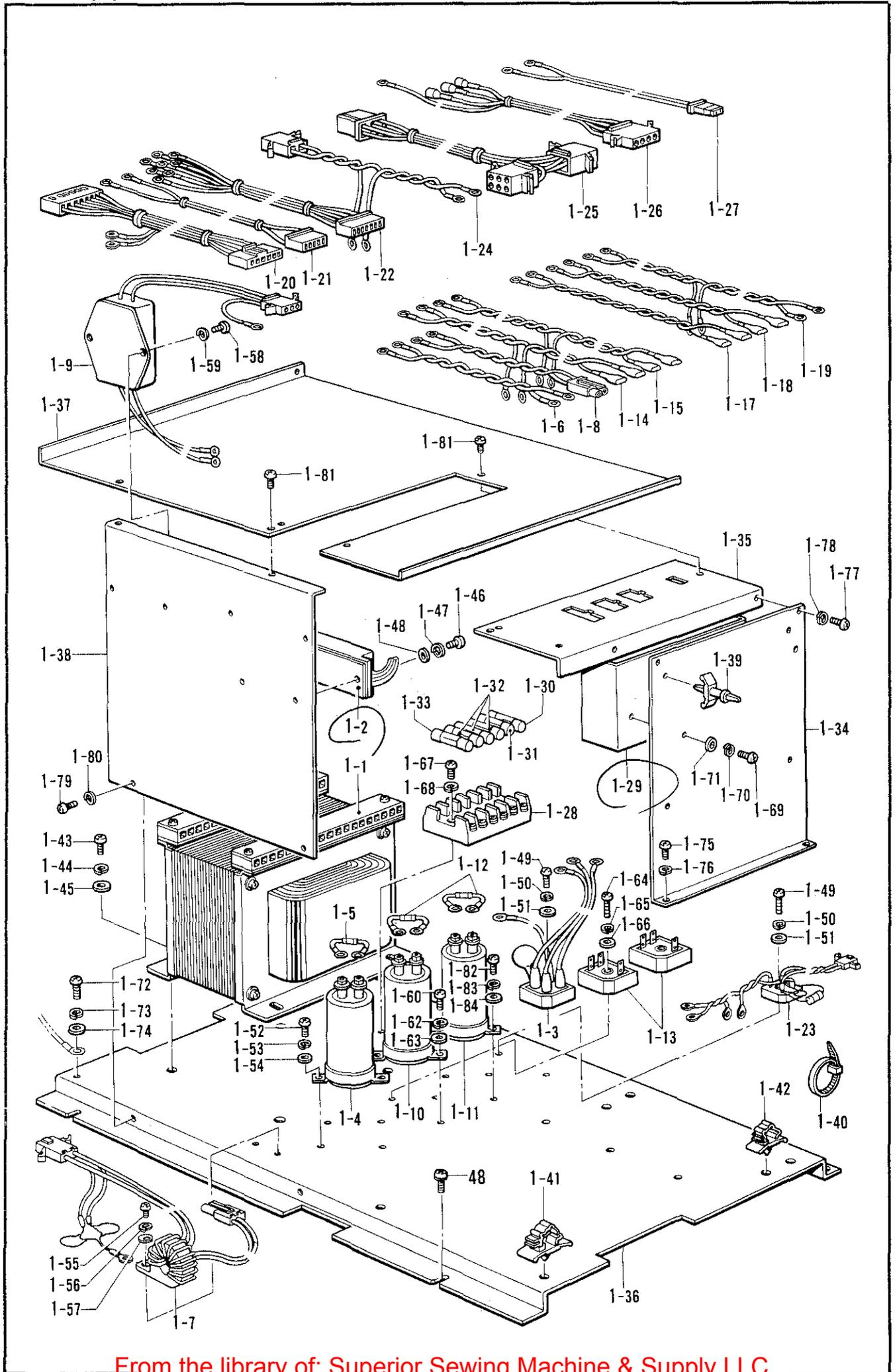
R1. 電装品関係/Power supply equipment mechanism/Stromversorgung/Mécanisme
