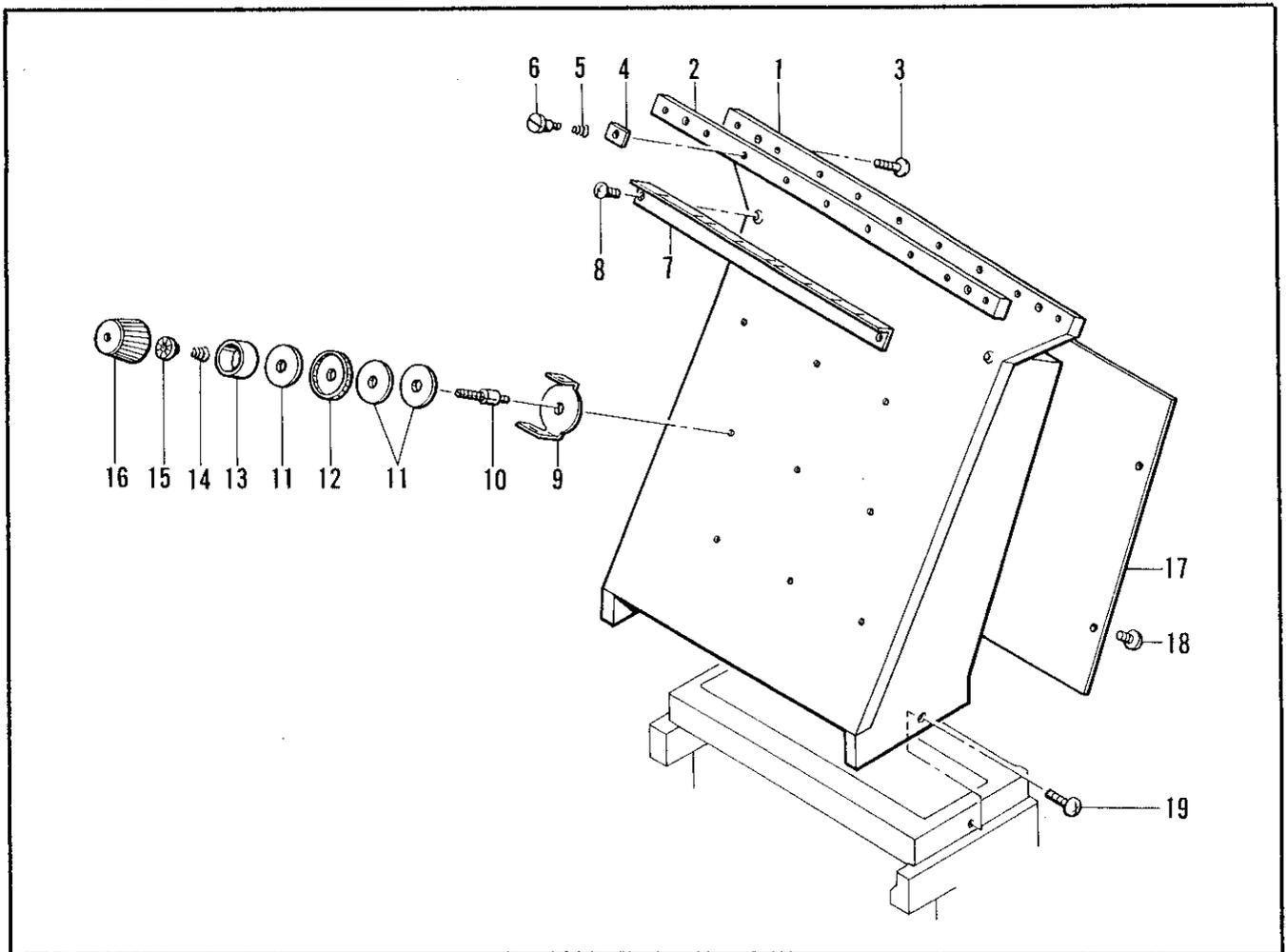
H. 上軸関係 / Upper shaft mechanism / Obere Welle /
